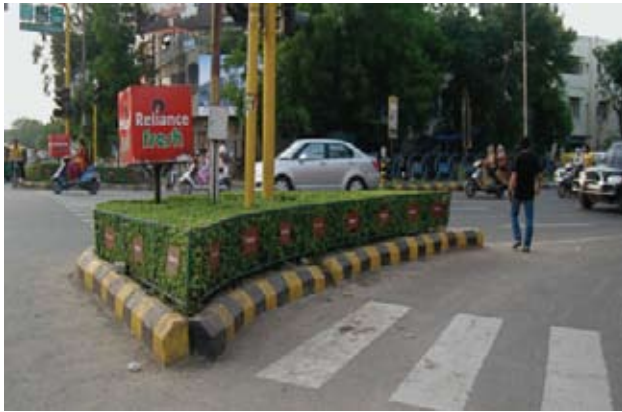
Figure 25: Islands That are Blocked with Fences or Planted With Vegetation are not Accessible to Pedestrians.
